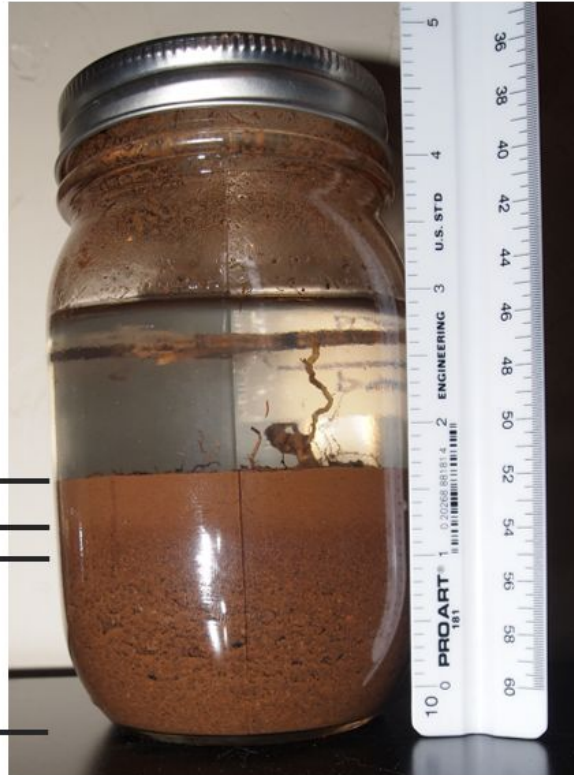
Figure 24: Jar test with soil sample #2 used to determine soil type
