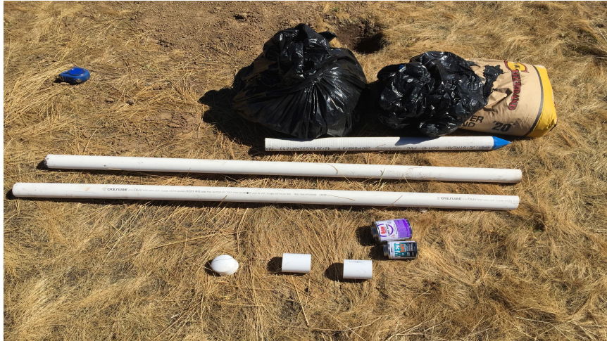
Figure 2: Monitoring well components
