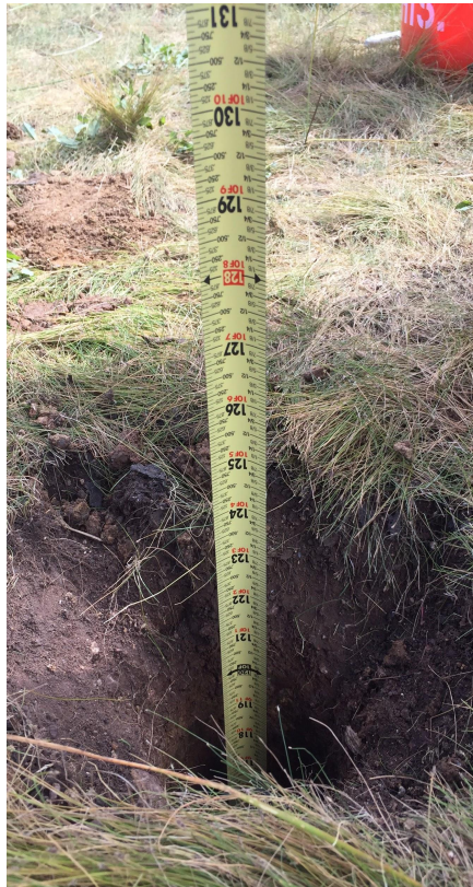
Figure 4: Augered hole measuring 126 inches
